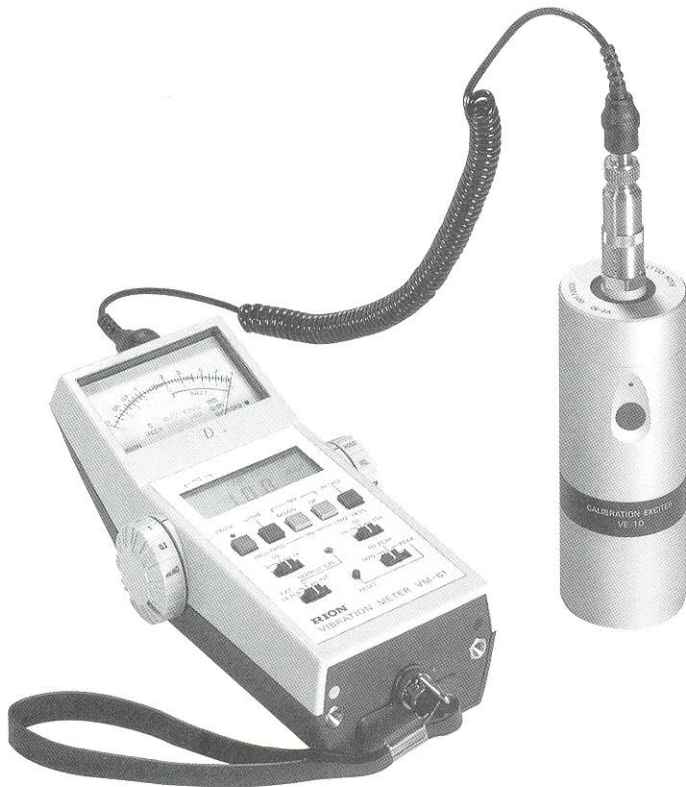
Calibration of Vibration Meter VM-61 by VE-10
