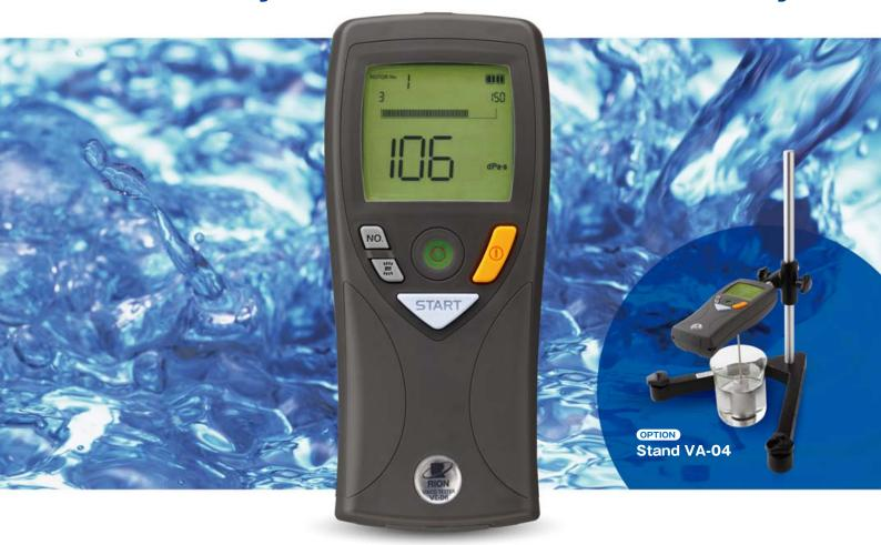
The VT-06 is designed for quality control applications in the manufacturing process of industrial products such as petrochemicals, paint, and adhesives, as well as foodstuffs. Viscosity measurements covering a wide range are possible, such as gear oil used in construction machinery. Measurement is performed by simply submerging a rotor in the fluid. The resistance to rotor movement caused by the viscosity (torque) is measured to obtain direct readings.
